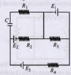
23. A part of ciucuit in a steady state along with the currents flowing in the branches, the values of resistances etc., is shown in the figure. Calculate the energy stored in the capacitor  $C(4\mu\text{F})$  [1986 - 4 Marks]
