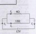
$$R_{\text{eq}} = \frac{R_1 R_2}{R_1 + R_2} = \frac{(6\Omega)(12\Omega)}{6\Omega + 12\Omega} = 4\Omega$$
