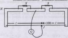
For a meter bridge at null point or at balanced condition
