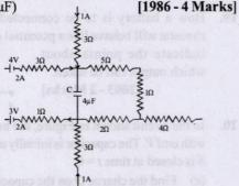
24. Calculate the steady state current in the 2-ohm resistor shown in the circuit in the figure. The internal resistance of the battery is negligible and the capacitance of the condenser C is 0.2 microfarad.
