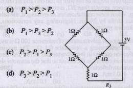
The three resistance of equal value are arranged in the different combinations shown below. Arrange them in increasing order of power dissipation. [2003S]
