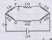
The resistance of the upper arm  $R_1 = 2\Omega + 2\Omega + 2\Omega = 6\Omega$
